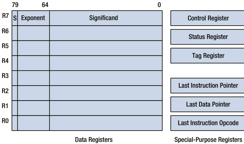
Figure 3-1. X87 FPU core architecture
