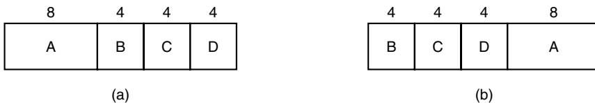
Figure 2-24. An example of shortest job first scheduling. (a) Running four jobs in the original order. (b) Running them in shortest job first order.
